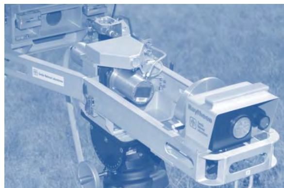
Low power version of the active denial system (ADS) technology
